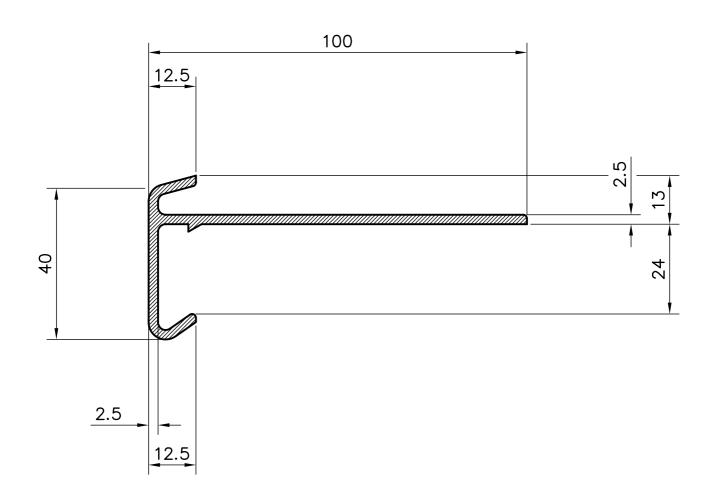
SUPPLIED IN 2.5 METRE LENGTHS WITH LOOSE JOINTING SLEEVE 90° INTERNAL AND EXTERNAL CORNER PIECES AVAILABLE STANDARD COLOURS BLACK, WHITE AND GREY OTHER COLOURS CAN BE SUPPLIED, PRICES & LEAD TIMES ON APPLICATION
