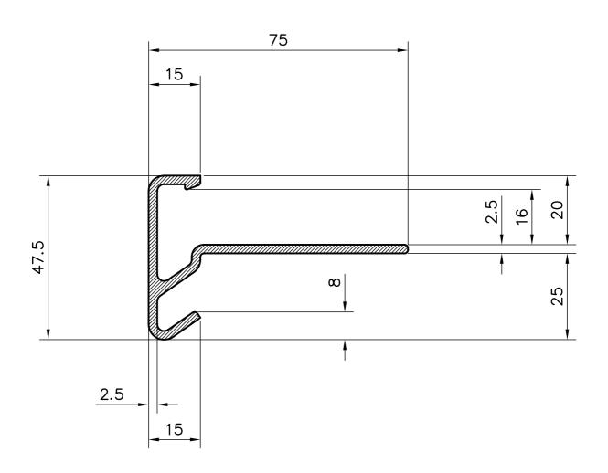
SUPPLIED IN 2.5 METRE LENGTHS WITH LOOSE JOINTING SLEEVE 90° INTERNAL AND EXTERNAL CORNER PIECES AVAILABLE STANDARD COLOURS BLACK, WHITE AND GREY OTHER COLOURS CAN BE SUPPLIED, PRICES & LEAD TIMES ON APPLICATION
